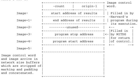
36-Bit Words Transmitted From MITDG's PDP-10 to Harvard's PDP-1
