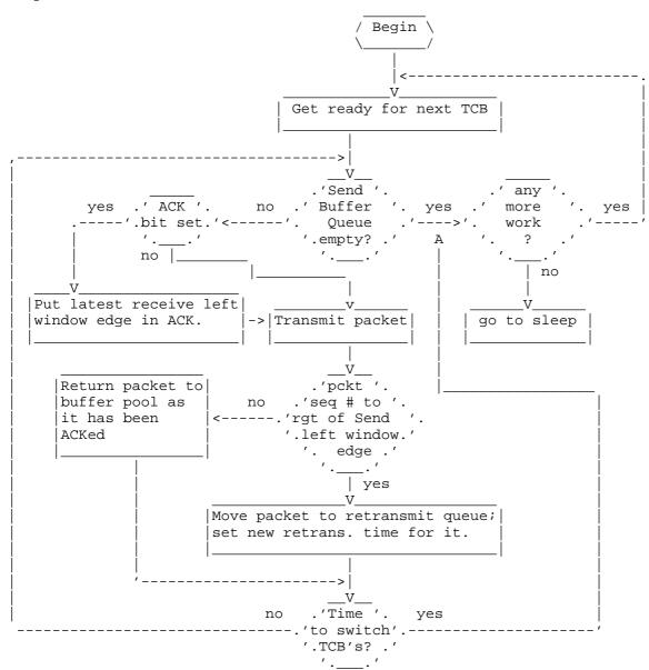
FIGURE 2.5b: Retransmit Process
