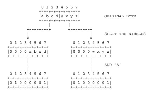
This encoding results in a NetBIOS name being represented as a sequence of 32 ASCII, upper-case characters from the set  $\{A,B,C...N,O,P\}$ .
