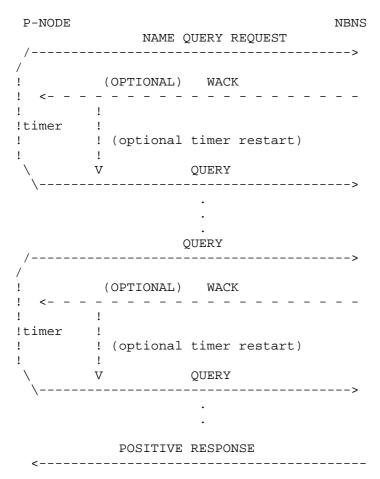
The following diagram illustrates NBNS redirection. Upon receipt of a NAME QUERY REQUEST, the NBNS redirects the client to another NBNS. The client repeats the request to the new NBNS and obtains a response. The diagram shows that response as a POSITIVE NAME QUERY RESPONSE. However any legal NBNS response may occur in actual operation.
