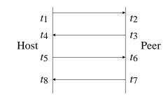
Figure 2. Calculating Delay and Offset
