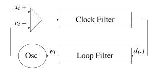
Figure 3. Phase-Lock Loop Model
