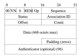
Figure 6. NTP Control Message Header
