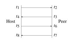
Figure 1. Calculating Delay and Offset
