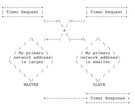
After link establishment, both sides of the link send Timer Request packets and start a timer waiting for a Timer Response. These Timer Requests are sent every 20 seconds until a response is received or a descision is made that the remote node is not responding. This could be after a predefined time (min. 60 seconds) or a number of retries (e.g., 16).
