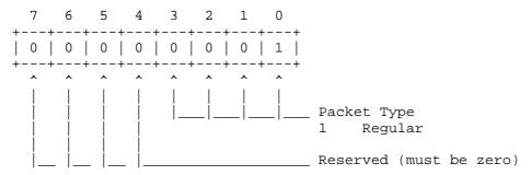
The Regular packet is rarely sent. Usually, the Regular packet is sent when there is not enough memory for the overhead of a new compression slot. Also, this type is included for future unforeseen changes to the IPX protocol which defeat the effectiveness of compression.
