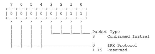
This type of packet is sent to inform the receiver to associate the IPX packet header with a slot number. This packet is sent each time a different header format is sent for a given slot, or when the sender has not received a Confirmation Packet from the receiver.
