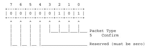
A Confirm Packet is exactly 3 octets in length. It consists of the
