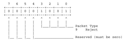
A Reject Packet is exactly 3 octets in length. It consists of the Flags, Slot Number and Rejected Flags fields.
