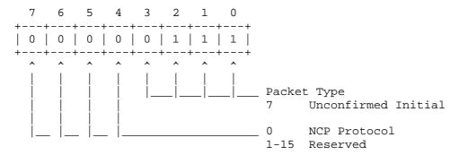
This type of packet is sent to inform the receiver to associate the IPX packet header with a slot number. This packet is sent each time a different header format is sent for a given slot.
