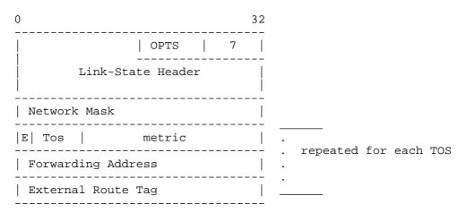
The definitions of the link-state ID, network mask, metrics and external route tag are the same as the definitions for the type-5 LSAs (see A.4.5 in the OSPF specification) except for:
