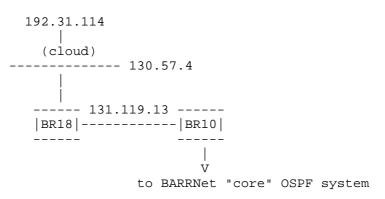
where the "cloud" consists of the subnets of 130.57 and network 192.31.114, all of which are learned by RIP on router BR18. Topologically, this cloud looks very much like an OSPF stub area. The advantages of running the cloud as an OSPF stub area are:
