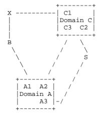
Given the domains, X, A, B, C and S, let domains A and C be running OSPF, and ASBRs A3 and C3 have equal cost multipath routes to A1, A2 and C1, C2 respectively. The picture above shows the internal structure of domains A and C only.
