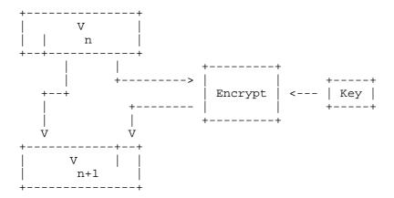
Note that if a shift of one is used, this is the same as the shift register technique described in Section 3 above but with the all important difference that the feedback is determined by a complex non-linear function of all bits rather than a simple linear or polynomial combination of output from a few bit position taps.
