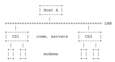
Assume that all of the modems are on the same rotary; that is, when a remote host dials in, it may be assigned a modem on either of the communication servers. Further assume that all of the remote hosts' IP addresses have the same subnet address as the servers and Host A, this in order to conserve address space.
