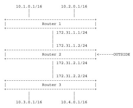
Router 1 can reach its two locally connected subnets, 10.1.0.0/16 and 10.2.0.0/16. It will aggregate them into a single announcement of 10.0.0.0/8 when it advertises out the 172.31.1.1 interface.
