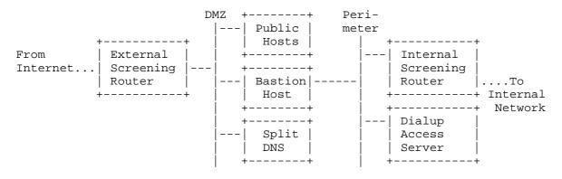
External screening routers typically have inbound access lists that block unauthorized traffic from the Internet, and outbound access lists that permit access only to DMZ servers and the bastion host. The inbound filters commonly block the Private Address Space, as well as address space from the enterprise's internal network. If the internal network address changes, the inbound filters clearly will need to change.
