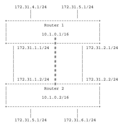
A common practice to provide router identifiers is using the "highest IP address" on the router as an identifier for the "box." Many implementations have a default mechanism to establish the router ID, which may be the highest configured address, or the highest active address.
