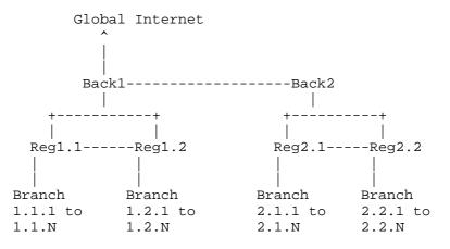
In this drawing, assume Back1 and Back2 exchange full routes; Back1 is also the exterior router. Regional routers (Reg) exchange full routes with one another and aggregate addresses to the backbone routers. Branch routers default to regional routers.
