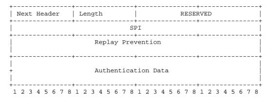
The Next Header, RESERVED, and SPI fields are specified in [RFC-1826]. The Length field is the length of the Replay Prevention field and the Authentication Data in 32-bit words.
