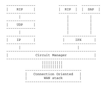
A WAN circuit manager will support a variety of network layer protocols, on its upper interface. On its lower interface, it may support one or more subnetworks. A subnetwork may support a number of Virtual Circuits.
