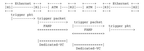
Figure 1. Trigger packet and FANP initiation
