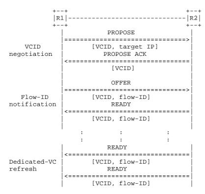
Figure 2. Flow ID notification and refresh procedure
