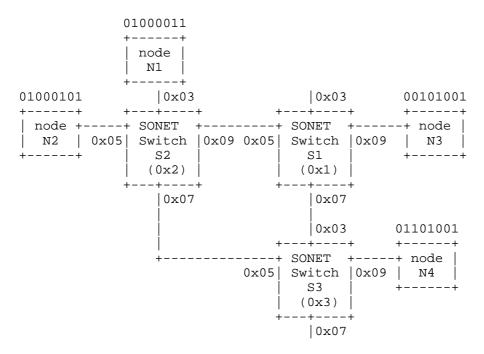
Figure 2 Multiple SONET Switch Environment
