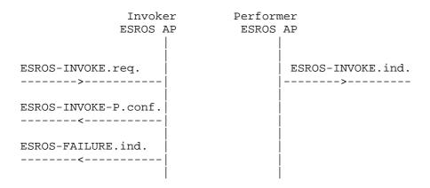
Figure 3: Time sequence diagram for ESROS-INVOKE service
