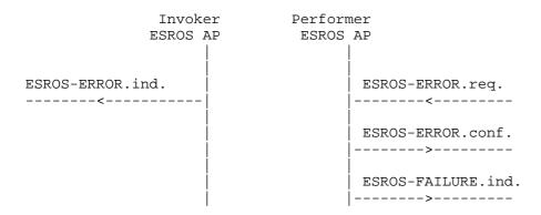
Figure 5: Time sequence diagram for ESROS-ERROR service
