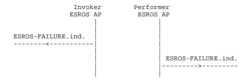
Figure 6: Time sequence diagram for ESROS-FAILURE service
