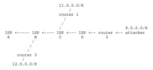
In the example above, the attacker resides within 9.0.0.0/8, which is provided Internet connectivity by ISP D. An input traffic filter on the ingress (input) link of "router 2", which provides connectivity to the attacker's network, restricts traffic to allow only traffic originating from source addresses within the 9.0.0.0/8 prefix, and prohibits an attacker from using "invalid" source addresses which reside outside of this prefix range.
