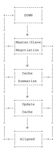
Figure 2: Cache Alignment Finite State Machine
