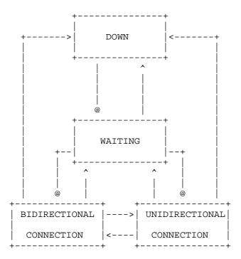
Figure 1: Hello Finite State Machine (HFSM)
