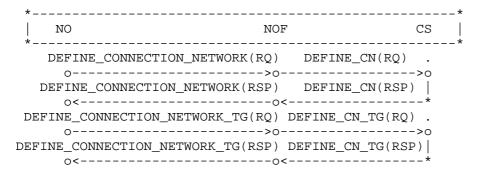
Figure 7. IP Connection Network Definition
