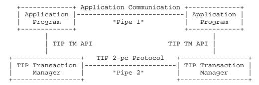
Fig 1: The two-pipe nature of TIP
