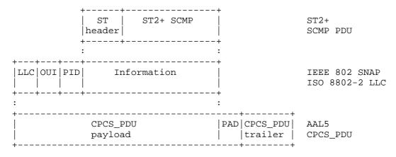
Fig. 6.2: RFC 1483 base encapsulation.
