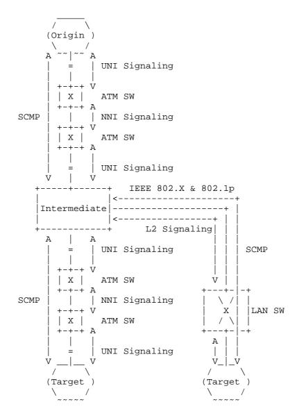
Fig. 2.6: Example of ST2+ SCMP interworking.
