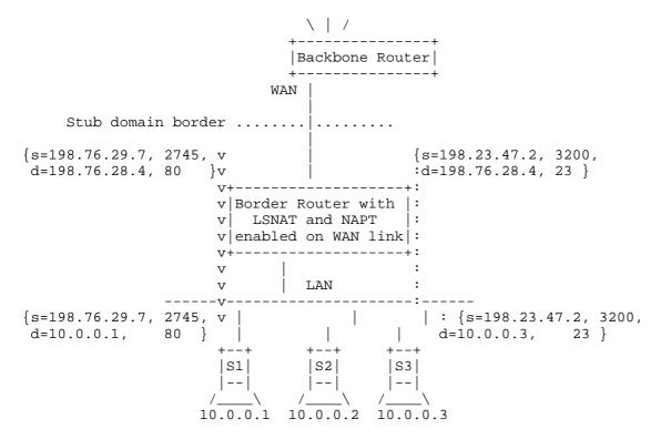
Figure 2: Operation of LSNAT, in coexistence with NAPT
