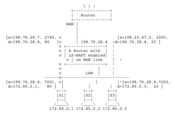
Figure 3: LS-NAPT configuration on a router
