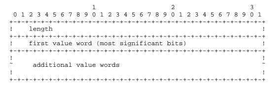
An example of such an encoding is given below, for a number with 51 bits of significance. The length field indicates that 2 32-bit quantities follow. The most significant non-zero bit of the number is in bit 13 of the first 32-bit quantity, the low order bits are in the second 32-bit quantity.
