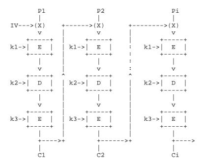
To decrypt, the order of the functions is reversed: decrypt with k3, encrypt with k2, decrypt with k1, and XOR with the previous ciphertext block.
