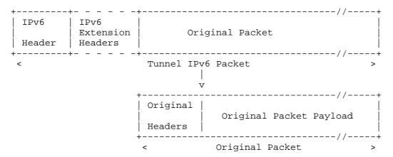
Fig. 4 Decapsulating a Packet
