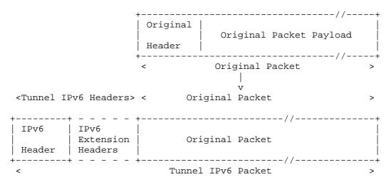
Fig. 3 Encapsulating a Packet
