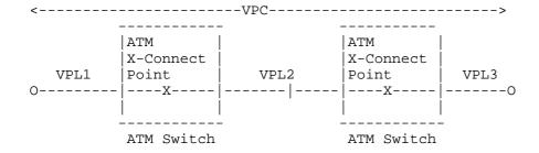
Figure 2: Virtual Path Links and Virtual Path Connection
