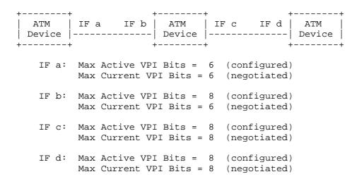
(between IF a and IF b, the minimum of the two configured "Max Active VPI Bits" is 6, so both interfaces set their "Max Current VPI Bits" to 6. Since IF c and IF d both are configured with "Max Active VPI Bits" of 8, they set their "Max Current VPI Bits" to 8.)
