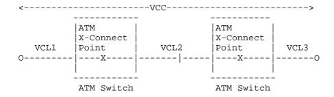
Figure 1: Virtual Channel Links and Virtual Channel Connection
