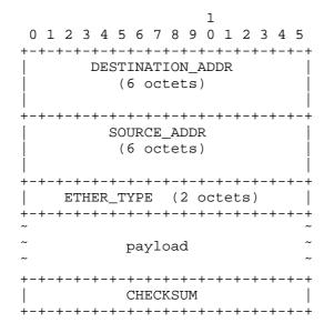
The DESTINATION\_ADDR field contains either a unicast Ethernet destination address, or the Ethernet broadcast address (0xffffffff). For Discovery packets, the value is either a unicast or broadcast address as defined in the Discovery section. For PPP session traffic, this field MUST contain the peer's unicast address as determined from the Discovery stage.
