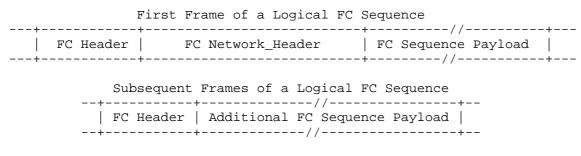
Fig. 2 FC Network\_Header in a Frame Sequence
