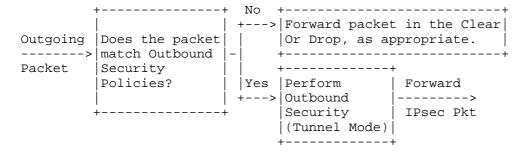
Figure 1. Operation of Tunnel-Mode IPsec on outgoing packets.
