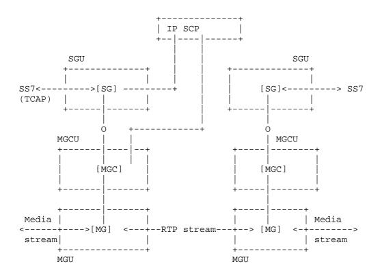
Figure 5: TCAP Signaling over IP
