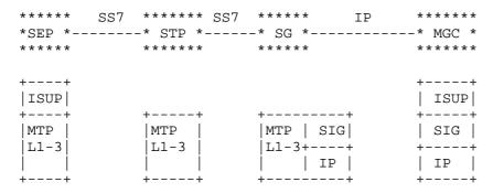
STP - Signal Transfer Point SEP - Signaling End Point SG - Signaling Gateway SIG - Signaling Transport MGC - Media Gateway Controller
