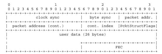
The two-byte Clock Synchronization and one-byte Byte Synchronization are located at the beginning of every scan line containing a NABTS packet and are used to synchronize the decoding sampling rate and byte timing.
