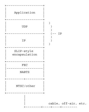
These protocols can be described in a bottom up component model using the example of NABTS carried over NTSC modulation as follows:
