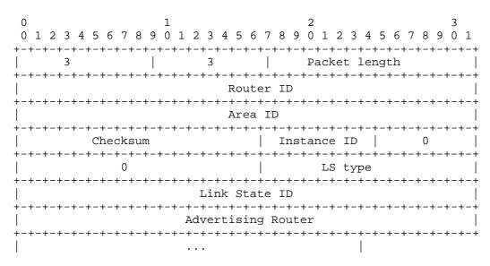
Each LSA requested is specified by its LS type, Link State ID, and Advertising Router. This uniquely identifies the LSA, but not its instance. Link State Request packets are understood to be requests for the most recent instance (whatever that might be).
