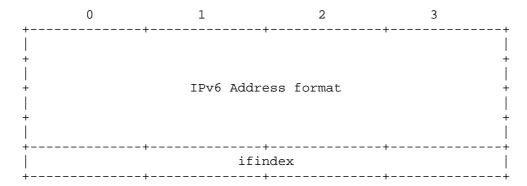
For this type of the interface object, the IPv6 address specifies the IP address that the incoming message came from. The ifindex is used to refer to the MIB-II defined local incoming interface on the PEP as described above.
