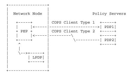
Figure 2: Multiple PDPs illustration.
