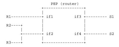
Figure 2: Multicast example: a single PEP view
