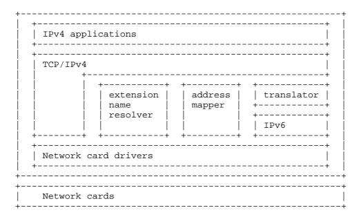
Figure. 1 Structure of the proposed dual stack host
