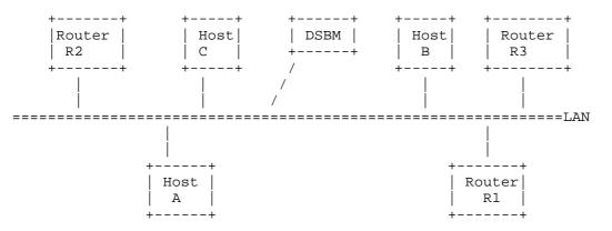
Figure 1 shows an example of a managed segment in a L2 domain that interconnects a set of hosts and routers. For the purpose of this discussion, we ignore the actual physical topology of the L2 domain (assume it is a shared L2 segment and a single managed segment represents the entire L2 domain). A single SBM device is designated to be the DSBM for the managed segment. We will provide examples of operation of the DSBM over switched and shared segments later in the document.
