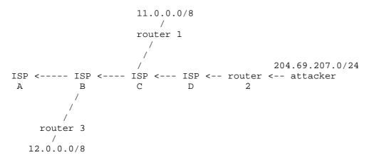
In the example above, the attacker resides within 204.69.207.0/24, which is provided Internet connectivity by ISP D. An input traffic filter on the ingress (input) link of "router 2", which provides connectivity to the attacker's network, restricts traffic to allow only traffic originating from source addresses within the 204.69.207.0/24 prefix, and prohibits an attacker from using "invalid" source addresses which reside outside of this prefix range.
