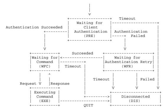
Figure 1: RRP Server Finite State Machine
