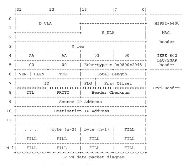
As shown in above figure the first eight bytes of the IP Datagram occupy the last eight bytes of the HIPPI-6400-PH [1] Header micropacket.
