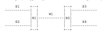
E1, E2, E3, and E4 are Ethernet LANs (or Token Ring, FDDI, etc.). W1 is a WAN (PPP over T1). B1 and B2 are MAC level bridges.
