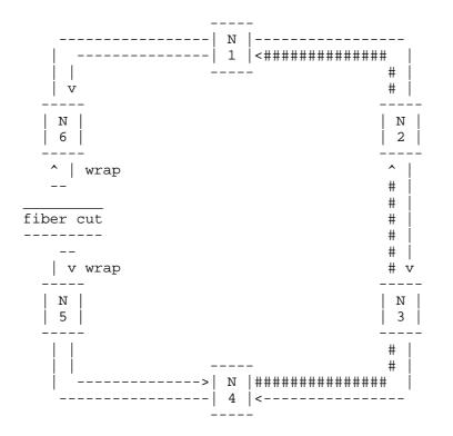
FIGURE 6. Data path after the new topology is discovered
