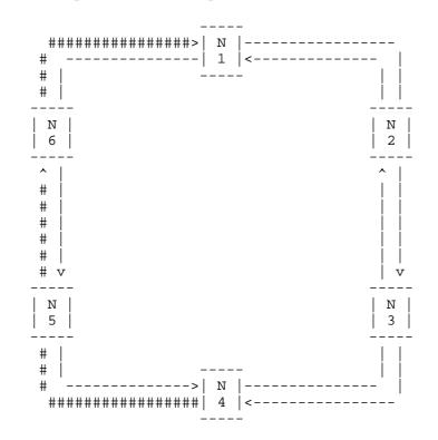
The ring wrap is controlled through SONET BLSR [3][4] style IPS signaling. It is an objective to perform the wrapping as fast as in the SONET equipment or faster.
