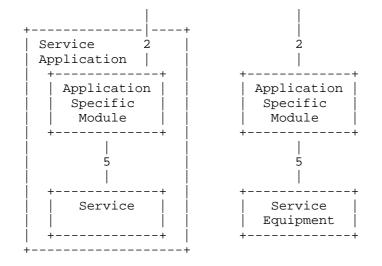
Fig. 4 -- ASM to Service Interaction (two views)
