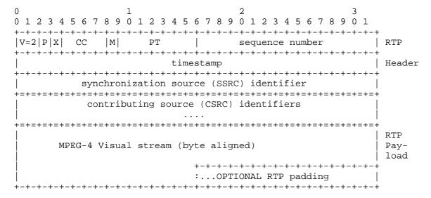
Figure 1 - An RTP packet for MPEG-4 Visual stream
