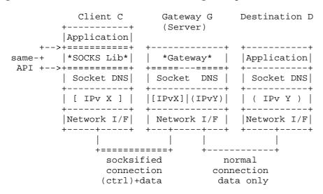
Fig. 1 Basic SOCKS-based Gateway Mechanism
