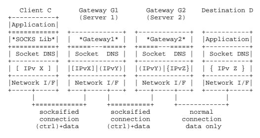
Fig. 2 Multiple Chained Relay Mechanism
