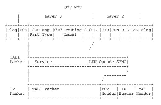
Figure 7: Encapsulation of ISUP MSUs using the TALI 'isot' opcode When an 'isot' TALI packet is received on an SG from an IP device, the SG performs the following processing on the 'isot' packet:
