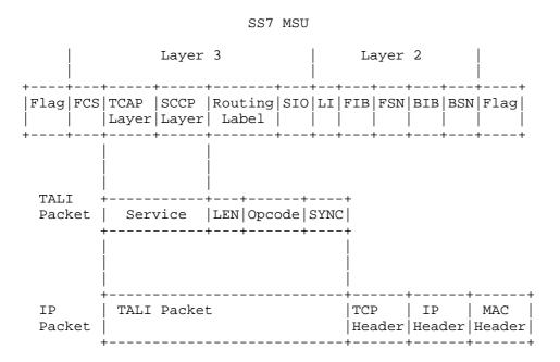
Figure 6: Encapsulation of SCCP MSUs using the TALI 'sccp' opcode When an 'sccp' TALI packet is received on by an SG from an IP device, the SG performs the following processing on the 'sccp' packet:
