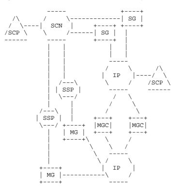
Figure 2: The Converged SS7 Network
