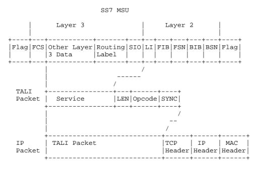
Figure 8: Encapsulation of SS7 MSUs with SI!=3,5,13 using 'mtp3'
