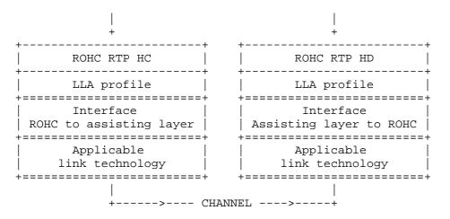
The figure above shows the various levels, as defined in [ROHC] and this document, constituting a complete implementation of the LLA profile. The figure also underlines the need for additional documents to specify how to implement these interfaces for a link technology for which this profile is relevant.
