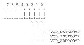
VCD\_DATACOMP: bit value 1. VCD\_INSTCOMP: bit value 2. VCD\_ADDRCOMP: bit value 4.
