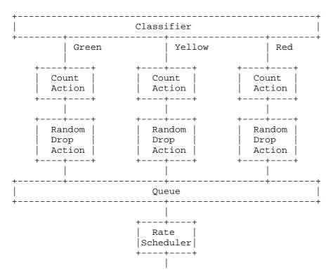
Figure 10: Typical AF Edge core interface configuration
