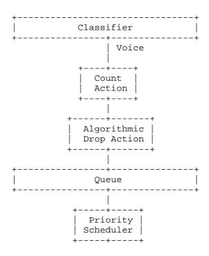
Figure 12: Typical EF Core interface Configuration
