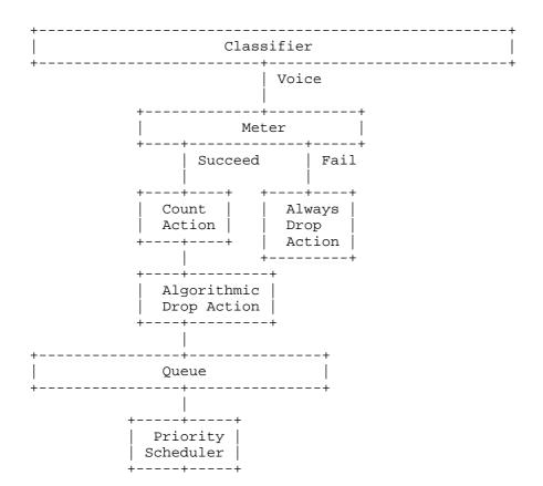
Figure 11: Typical EF Edge (Policing) Configuration
