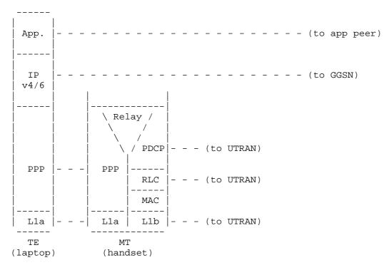
Figure 3: Laptop Attached to 3GPP Handset
