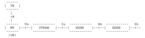
Figure 1: Simplified GPRS Architecture
