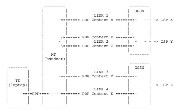
Figure 3: Correspondence of PDP Contexts to IPv6 Links
